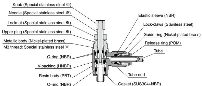
※ Equivalent Corrosion Resistance to SUS303
